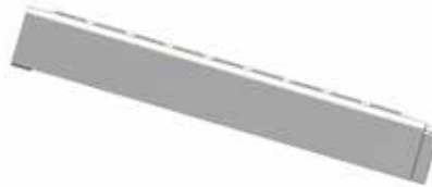
Array Skirt Roof pitch >2:12: Not required Roof pitch < 2:12: Required UL 1703 Fire and UL 2703 Tested & Certified Class A
