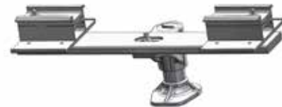
Double Mount UL 2703 Tested & Certified Tighten to 135 in-lbs
